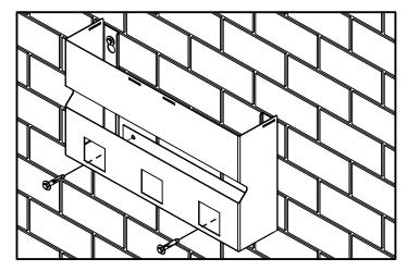
4. Fit two bolts through the lower holes in the back of the case. Now FULLY TIGHTEN ALL 4 BOLTS, checking that the unit is level.
