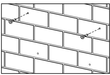
2. Drill four holes in the wall for the fixings as per the fixing manufacturers instructions and fit two fixings into the upper holes only.
