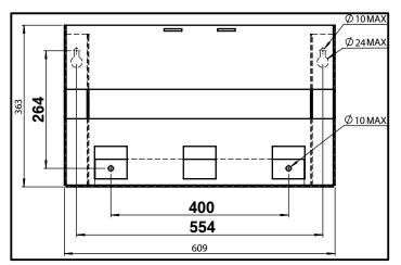
1. Hold the unit up to the wall, level the unit, and mark the position of the holes, or use the above fixings diagram. (A card template can also be used.)
