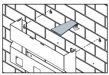
3. Hook the bayonet holes over the washers of the two upper bolts and tighten slightly. (these MUST be fully tightened shortly), this allows adjustments to be made when lining up the two lower bolts.
